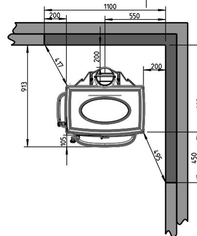
Min. distance to combustible wall protected by firewall
