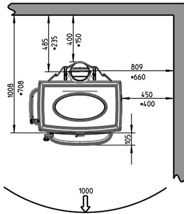
\* With heat shield rear and insulated flue pipe
